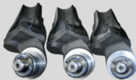
Drilling bit legs
