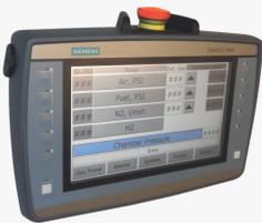
AK02: Wide-Screen Industrial Operator Tablet and Data Visualization System
